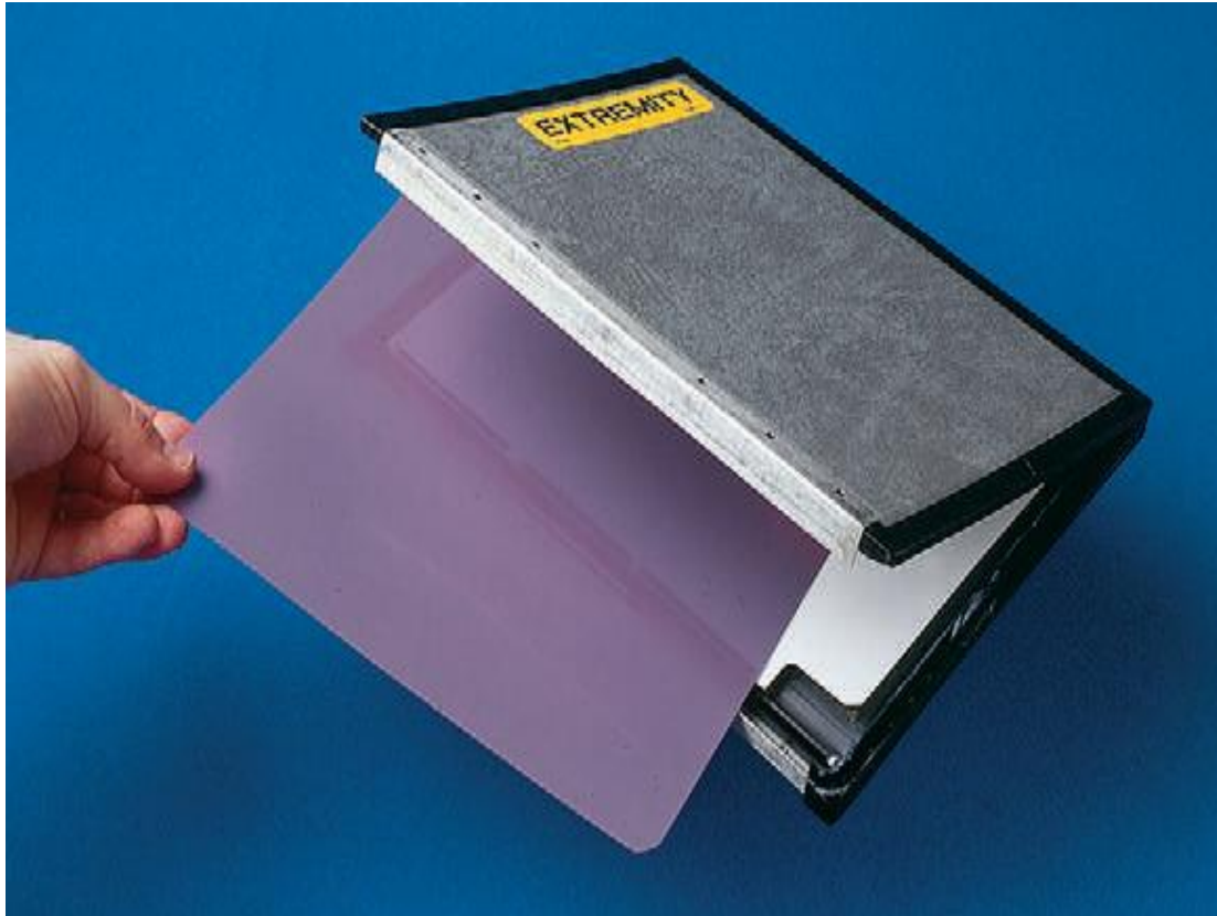
Image receptors. Conventional radiographic cassette, opened and showing a sheet of x-ray film.
