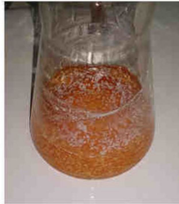
dark red precipitate of \text{AgSCN}
